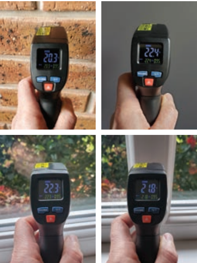
The thermometer can give you the difference in surface temperature between materials that have different thermal conductivity/insulation properties.
