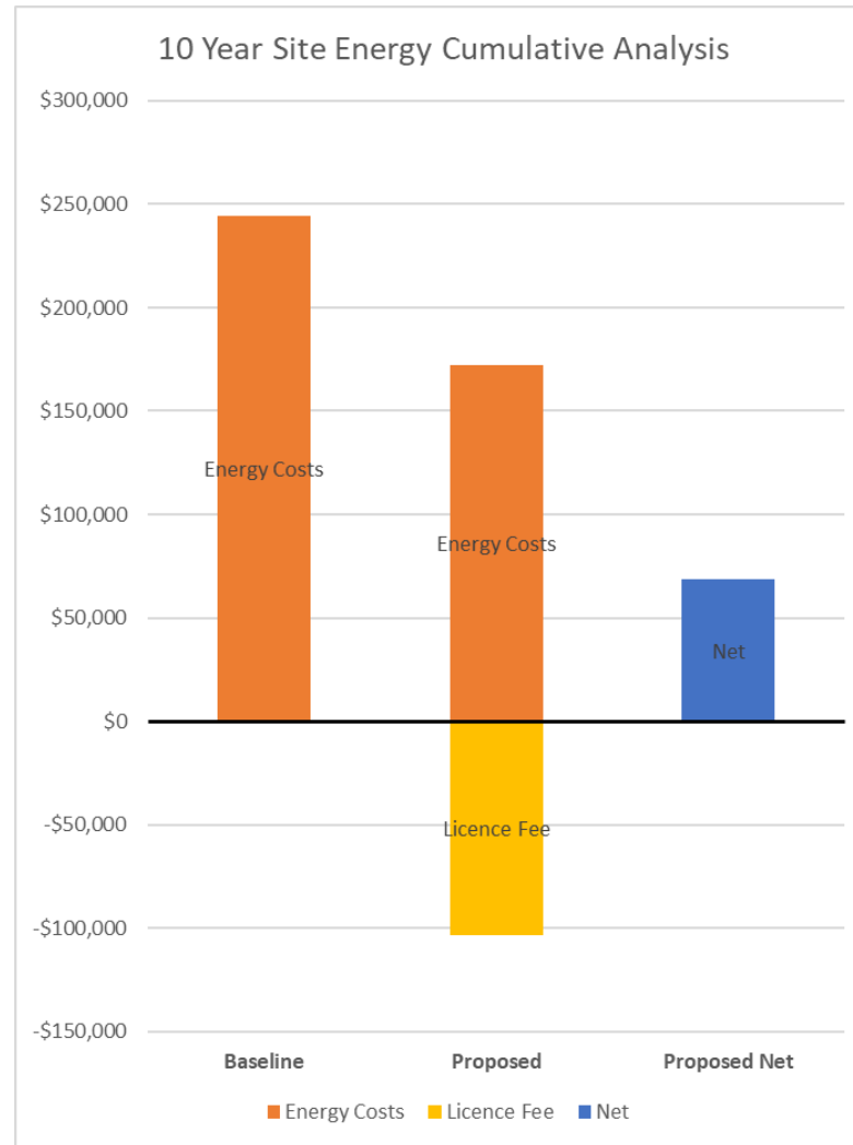
Figure Two. Ten year host site energy analysis under a scenario where Council owns the battery and licenses its use to Indigo Power.
