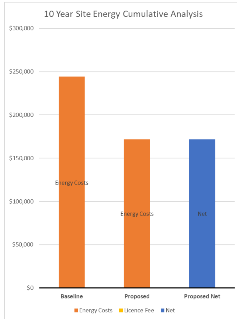
Figure One. Ten year host site energy analysis under a scenario where the battery is owned by Indigo Power, who leases an area of the site.
